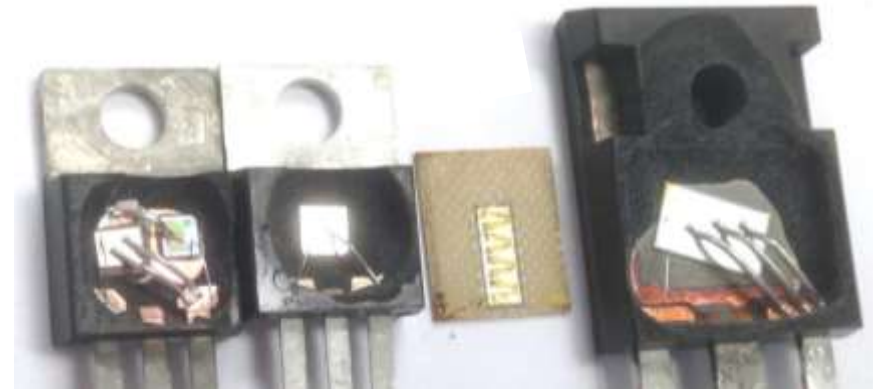
UJC6505T SCT2120AF GS66508B IPP65R045C7 Cascode SiC MOSFET GaN HEMT Si Superjunction
